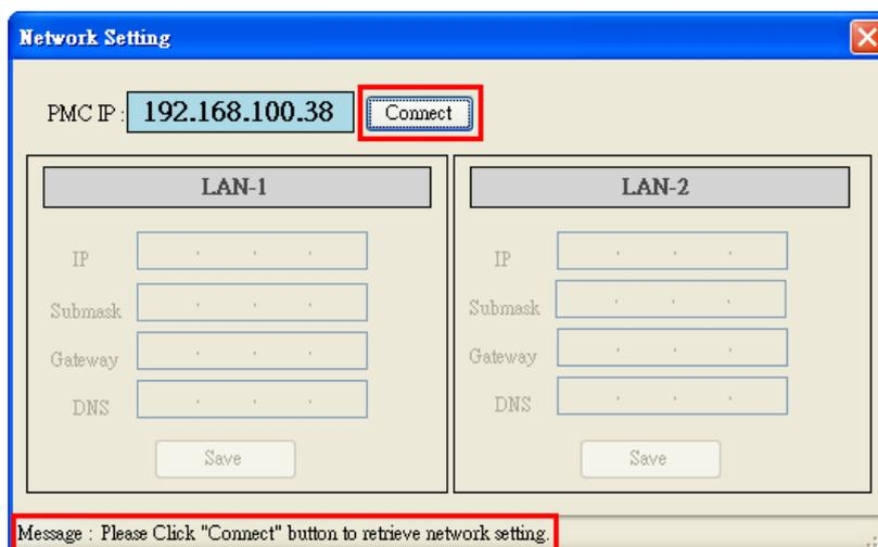
Click “Connect” button to retrieve the detailed network setting of the selected PMC. After modifying the settings of LAN1 or LAN2, please click “Save” button to update the network settings of the selected PMC.
